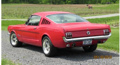
(disc brakes on the front and a dual diagonal master cylinder, lowered suspension, wheels, tires, Hurst shifter). It has no rust whatsoever. It's 53 years old, and driving it shows how cars have come a long way - the stock bucket seats provide no back support and it rides like a buckboard, appropriate for a car named Mustang!
